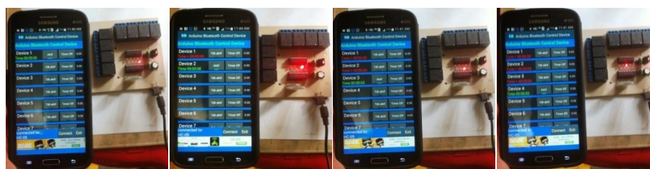
(a) Relay 1 ON (b) Relay 2 ON (c) Relay 3 ON (d) Relay 4 ON
