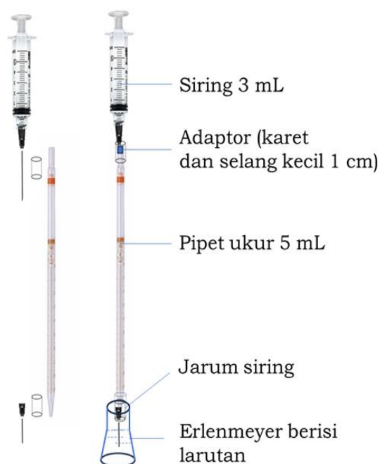
Gambar 2. Small Scale Chemistry Kit titrasi asam-basa skala mikro
