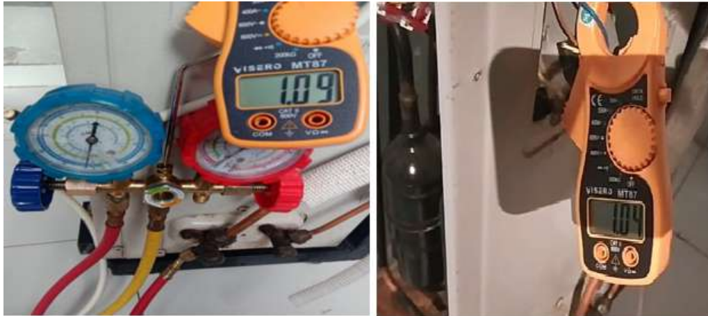
Gambar 5. Pengujian arus running AC split saat refrigeran kosong
