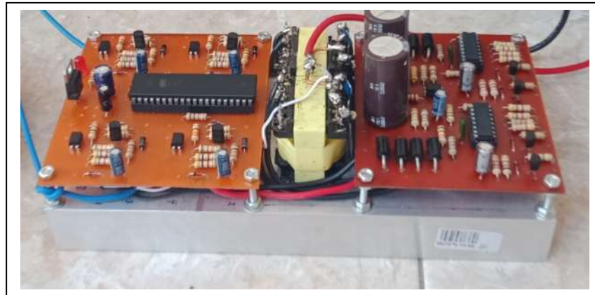
Gambar 5. Prototipe inverter cascaded H-bridge lima level berbasis mikrokontroler AT89S52
