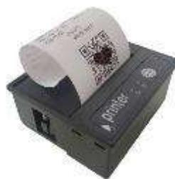
Gambar 8. *Thermal Printer*
